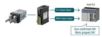
(3) Detect the presence of a load The position of the attachment when the load is gripped
